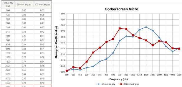
Plain & anodised panels are equivalent in absorption ested to ISO 354:2003 (reduced size reverberation room) eport Number: 23816AR
