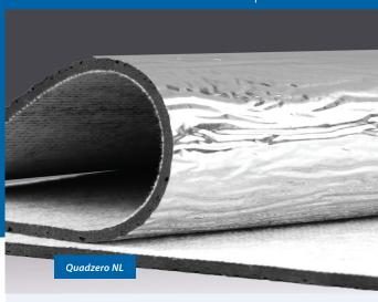
Quadzero™NL is a high performance foil faced mass loaded vinyl noise barrier, approved for use in maritime applications as a surface covering or veneer for bulkheads and ceilings, applied on top of marine certified insulation systems.
