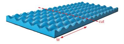
Pyrotek recommends an overlap at all joins to eliminate potential flanking noise. The removal of foam before overlapping at joints will provide a better acoustic seal and smooth surface
