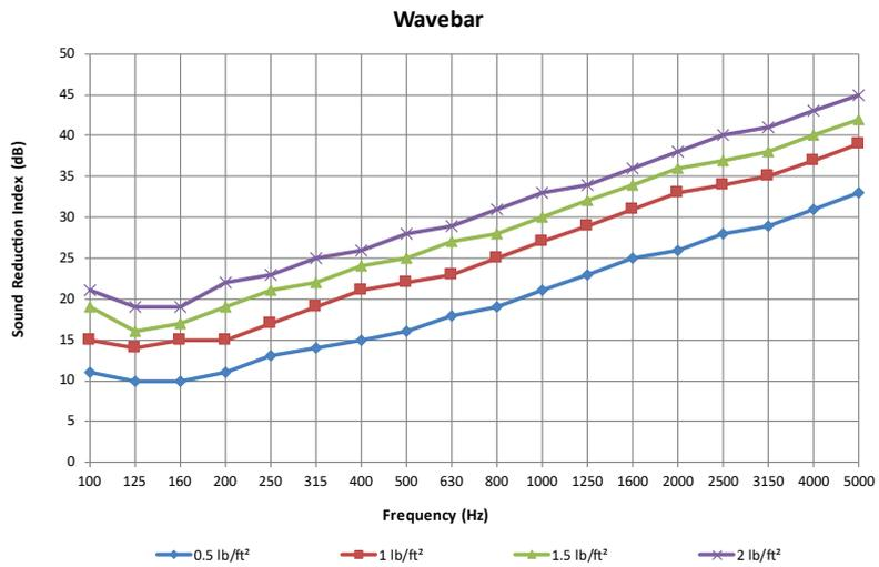
Tested to ASTM E90 at Riverbank Acoustical Laboratories, USA
