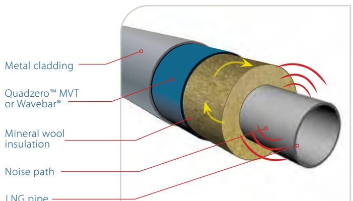
Wavebar® complies to the ISO 15665 (Group 2 Pipe size) test method.
