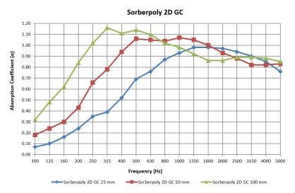
Tested to ISO 354:2003 at University of Canterbury, New Zealand | Report Numbers: 305, 306 & 346 Acoustic results are based on 32 kg/m³ density material
