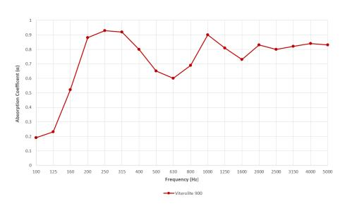
Tested to ISO 354:2003 at CSIRO, Australia | Report Number: AC323-01-1 The above results are based on the Viterolite® 900 rail track tile design
