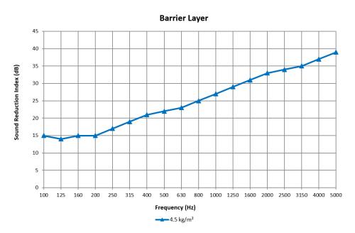
Tested to ASTM E90-09 at Riverbank Acoustical Laboratories, USA
