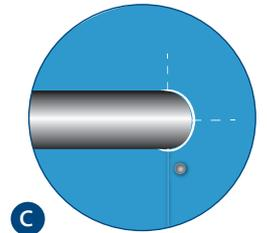
**c** ensure all junctions of ducting and wavebar are securely taped, mechanically fixed or sealed with plasticiser resistant mastic
