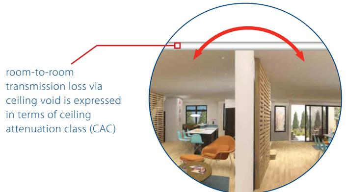
room-to-room transmission loss via ceiling void is expressed in terms of ceiling attenuation class (CAC)
