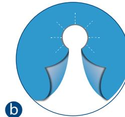
**b** move pipe or wavebar into location before closing flaps behind the pipe
