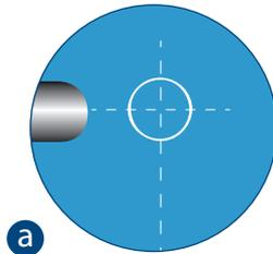
**a** cut a slit from edge of sheet to pipework location. cut flange lines to diameter of pipe
