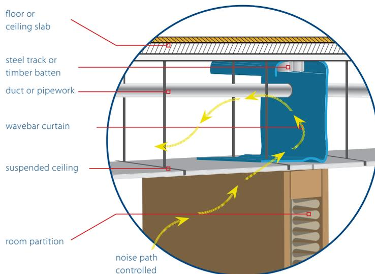
*Pyrotek's Wavebar® reduces crosstalk ceiling noise dramatically. Refer to 'Wavebar® TDS-311IP' for more information*
