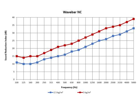
Tested to ASTM E90 at Riverbank Acoustical Laboratories, USA Report Numbers: TL18-641 & TL18-642
