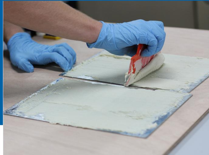
*Both parts are supplied in the required ratio of ingredients with a weight based mixing ratio of 10:1 of part A to B and must be mixed thoroughly before use.*
