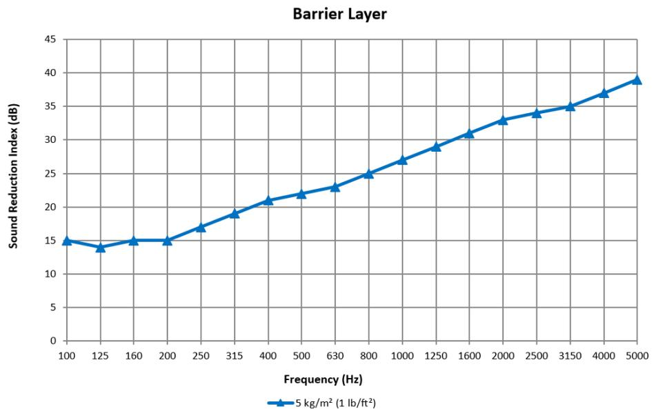
Tested to ASTM E90-09 at Riverbank Acoustical Laboratories, USA
