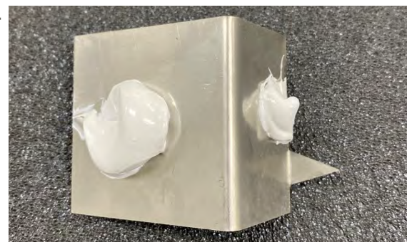
RB Centre Bracket with adhesive applied
