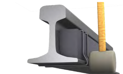
2b. Installing Decidamp RTD Clips
